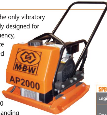
Further, the mechanical construction of the AP2000 is specific to this very demanding application. Stress relieved steel plate housings are crack resistant and provide long wear. Aluminum exciter housing dissipates heat rapidly and custom lubricants preserve bearing and seal integrity. The self cleaning plate prevents dirt build-up.
